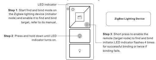
Note: Each remote can bind max. 30 lighting devices.
