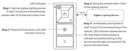
Note: 1) Directly TouchLink (both not added to a ZigBee network), each remote can link with 30 devices.
