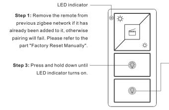
Step 2: From your zigbee controller or hub interface, choose to add device or accessory and enter Pairing mode as instructed by the controller.
